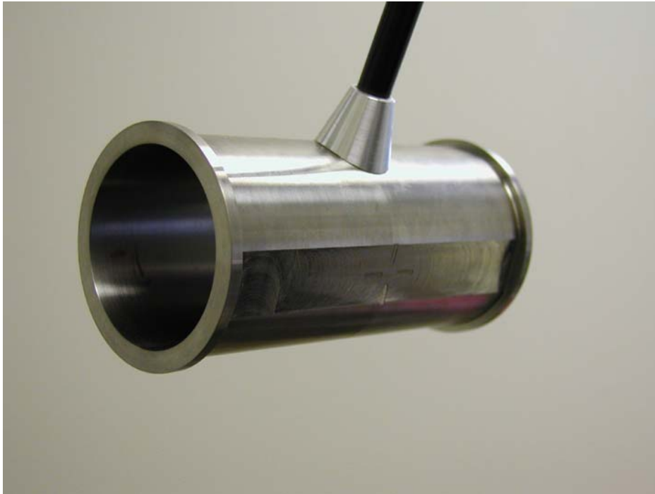
Figure 2: An image of a calibration club for use with the pendulum device.
