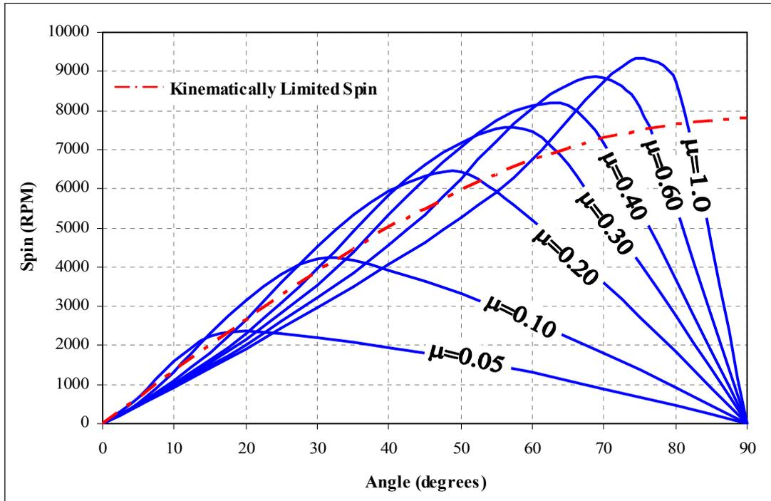
**Figure 9:** Effect of loft on model results for Pinnacle Gold (80 ft/s impact speed)
