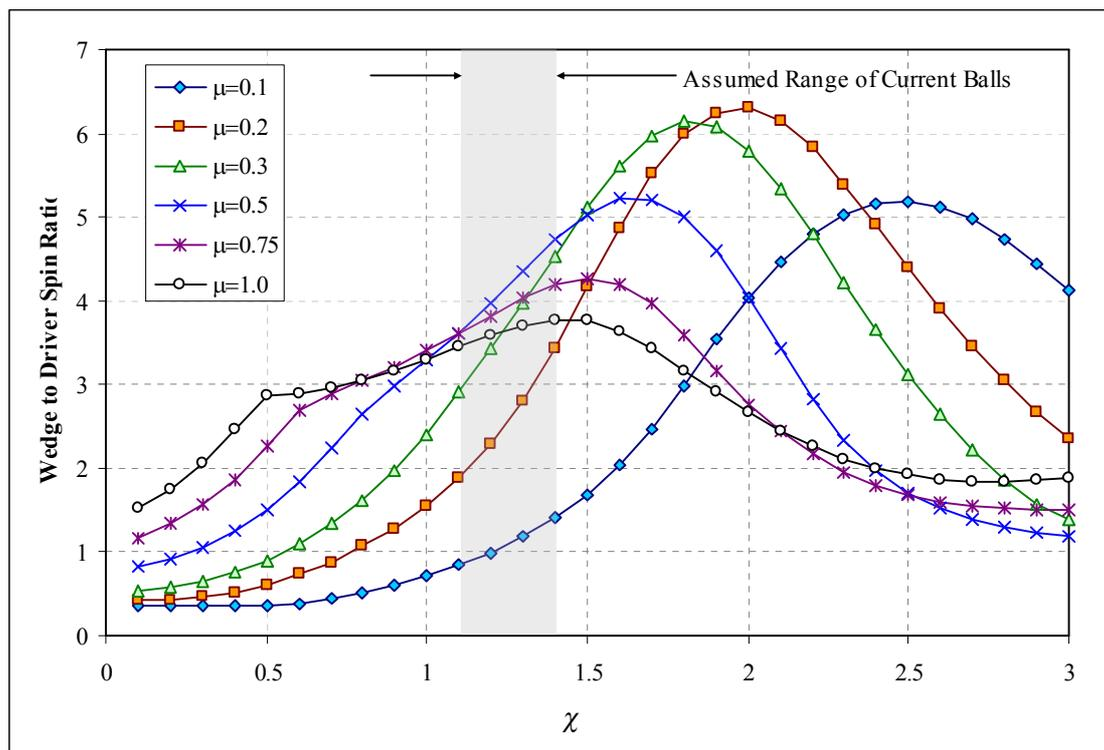
**Figure 11:** Effect of tangential flexibility on wedge/driver spin ratio
