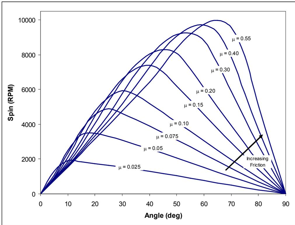
**Figure 7.2:** Effect of coefficient of friction on spin rate using Maw model
