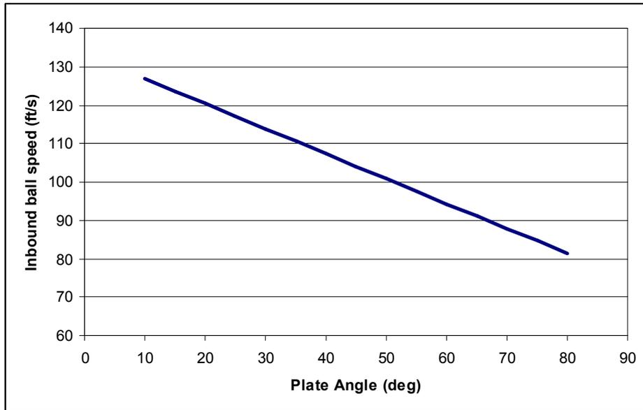
**Figure 6.3:** Inbound ball speed as a function of test plate angle
