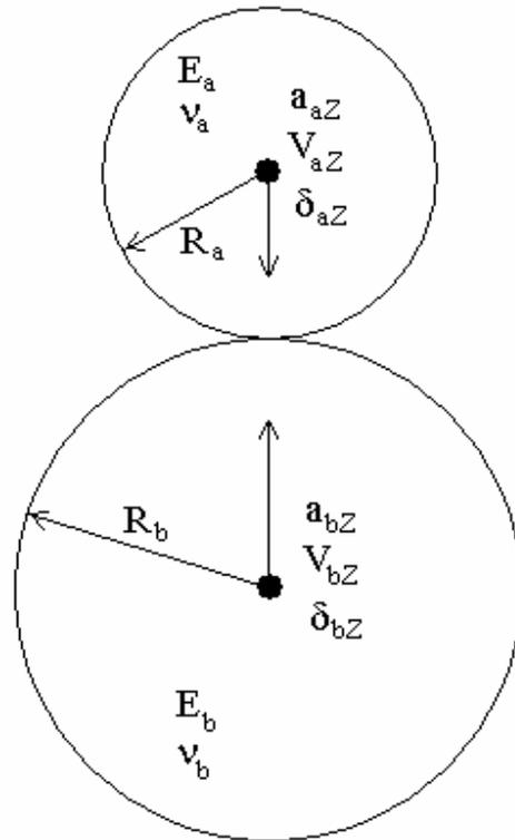
**Figure 1:** Normal contact of elastic spheres
