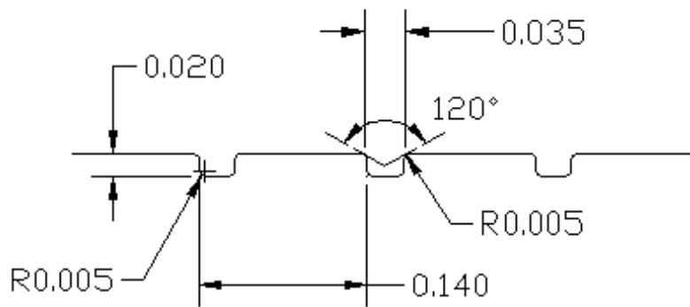
**Figure 4.1:** U-groove specification (all dimensions in inches and angles in degrees)
