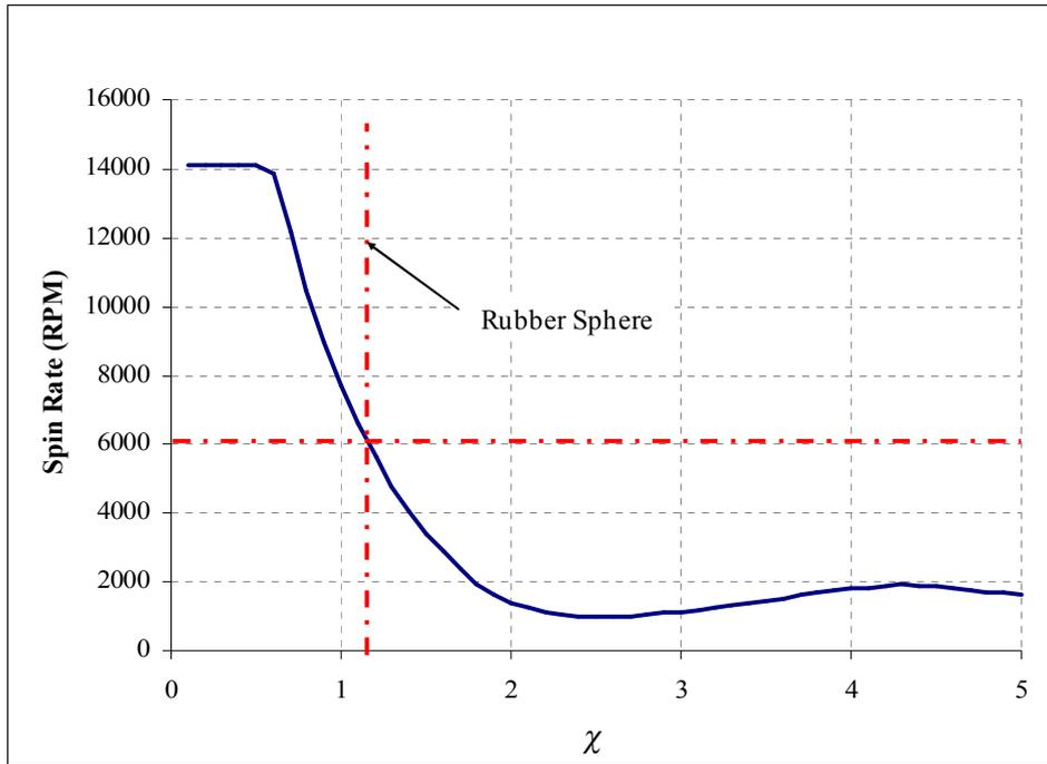
**Figure 4:** Effect of tangential stiffness on spin rate (30° barrier, 80 ft/s,  $\mu=0.3$ )
