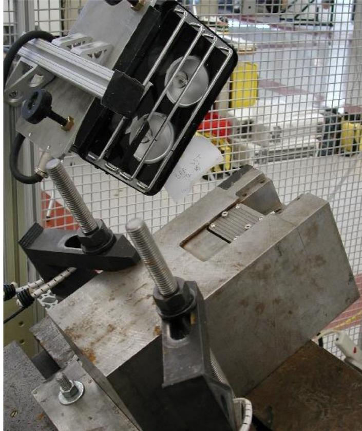
**Figure 3:** Grooved test plate oblique impact test setup
