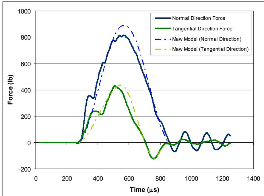
**Figure 7.1:** Typical comparison of measured and predicted force time histories (60 degree plate angle)
