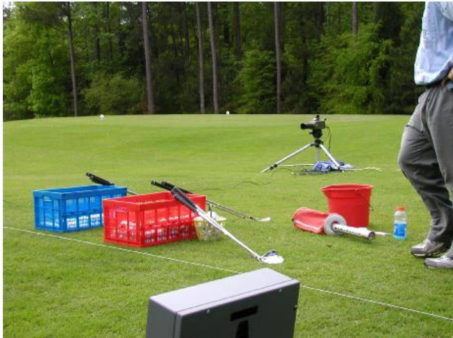
**Figure 3b** – Close-up of Test Set-up showing High Speed Video, Radar and Test Equipment
