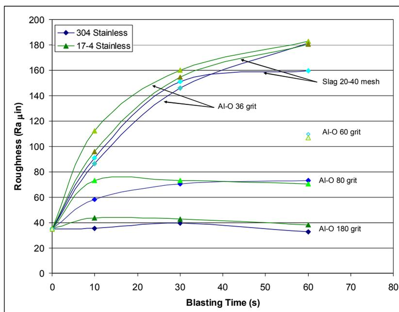
**Figure 4.5:** Abrasive blasting results
