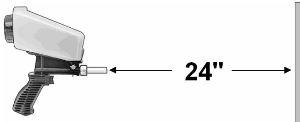
**Figure 1:** Abrasive blasting schematic
