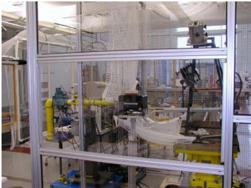
**Figure 2 – Spin Test Set-up**
