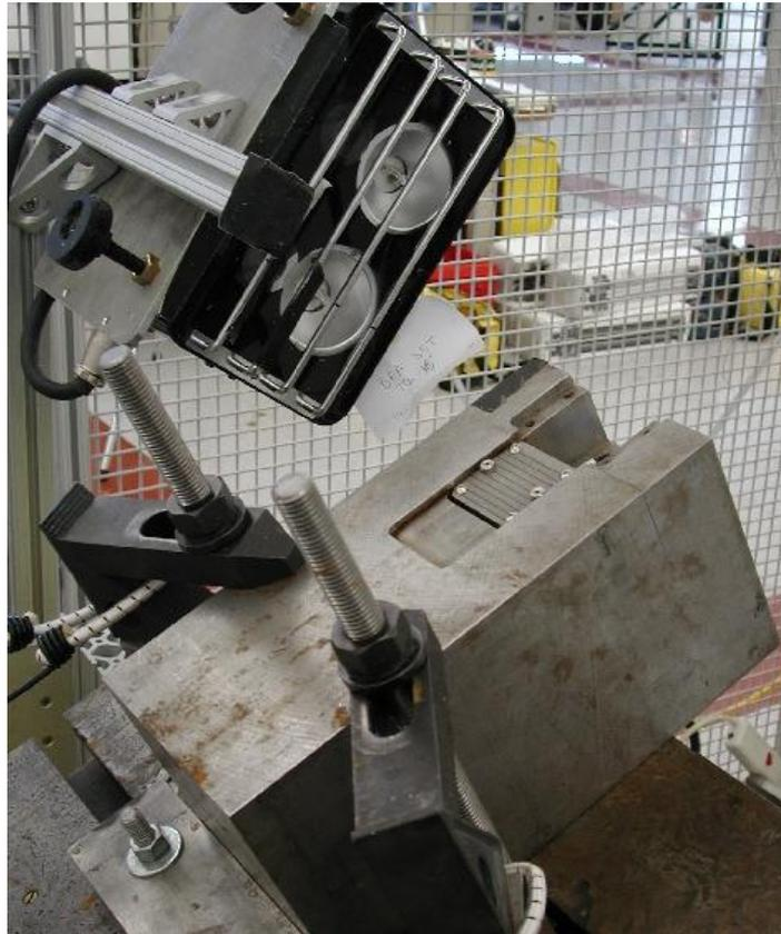
**Figure 3:** Grooved test plate oblique impact test setup
