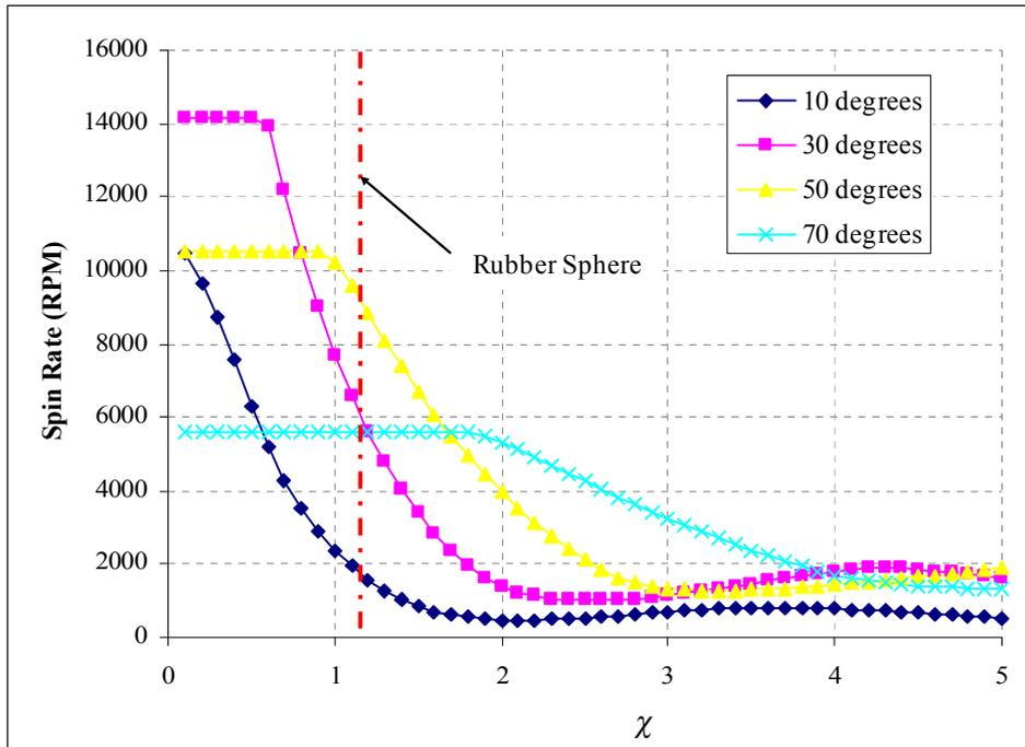
**Figure 5:** Effect of tangential stiffness and impact angle on spin rate (80 ft/s,  $\mu=0.3$ )
