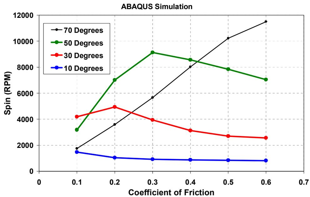
**Figure 7**– Results of Simulations of Oblique Impacts at Various Friction Levels
