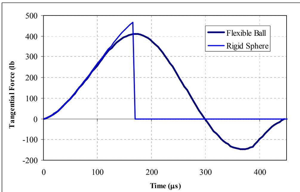
**Figure 2:** Tangential force history for tangentially flexible and rigid spheres ( $30^\circ$  barrier, 80 ft/s,  $\mu=0.3$ )
