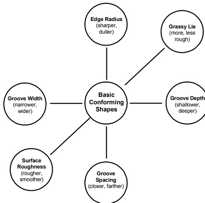
**Figure 3.1:** Plate testing experimental parameters
