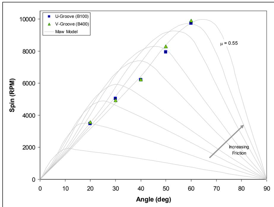
**Figure 8.2:** Comparison of spin rate in dry conditions (U and V groove plates) to Maw model
