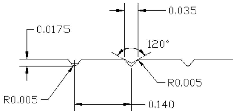
**Figure 4.2:** V-groove specification (all dimensions in inches and angles in degrees)
