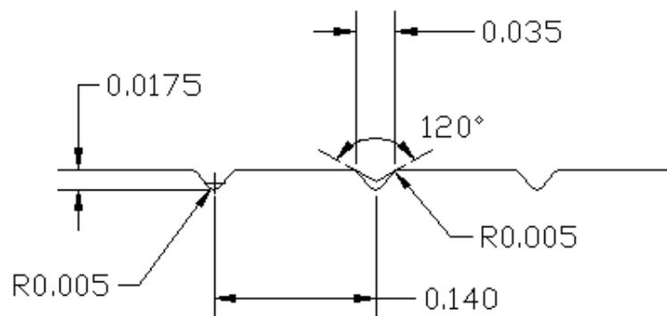
**Figure 1 – V-groove Specifications**
