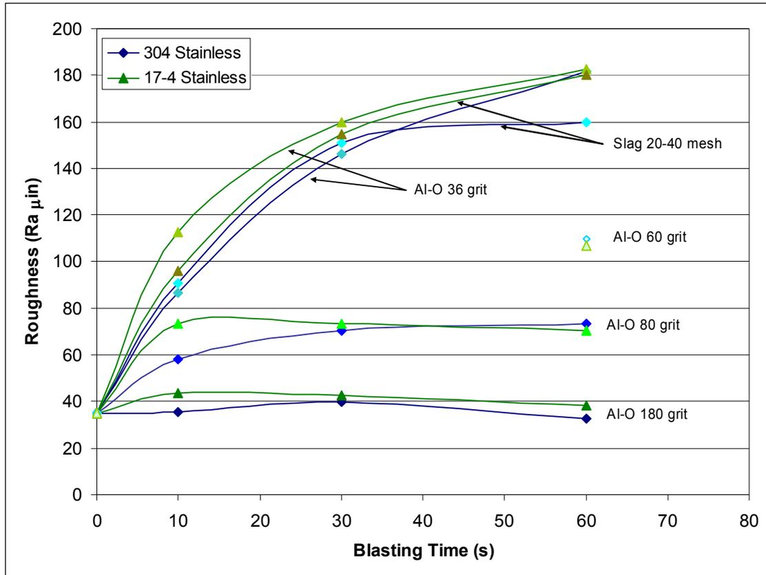
**Figure 2:** Surface roughness results ( $\diamond$  - 304 stainless steel,  $\blacktriangle$  - 17-4 stainless steel)
