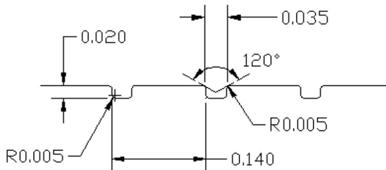
**Figure 2 – U-groove Specifications**
