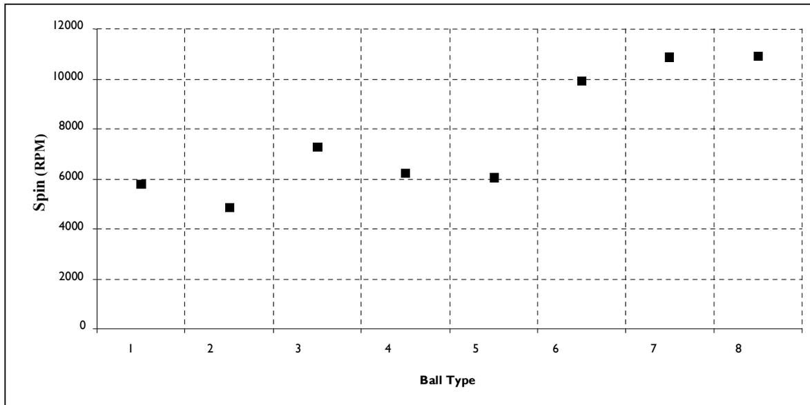
**Figure 6.5:** Spin as a function of ball type following impact with B100 grooved plate under dry conditions at 100 ft/s at a loft angle of 60°.
