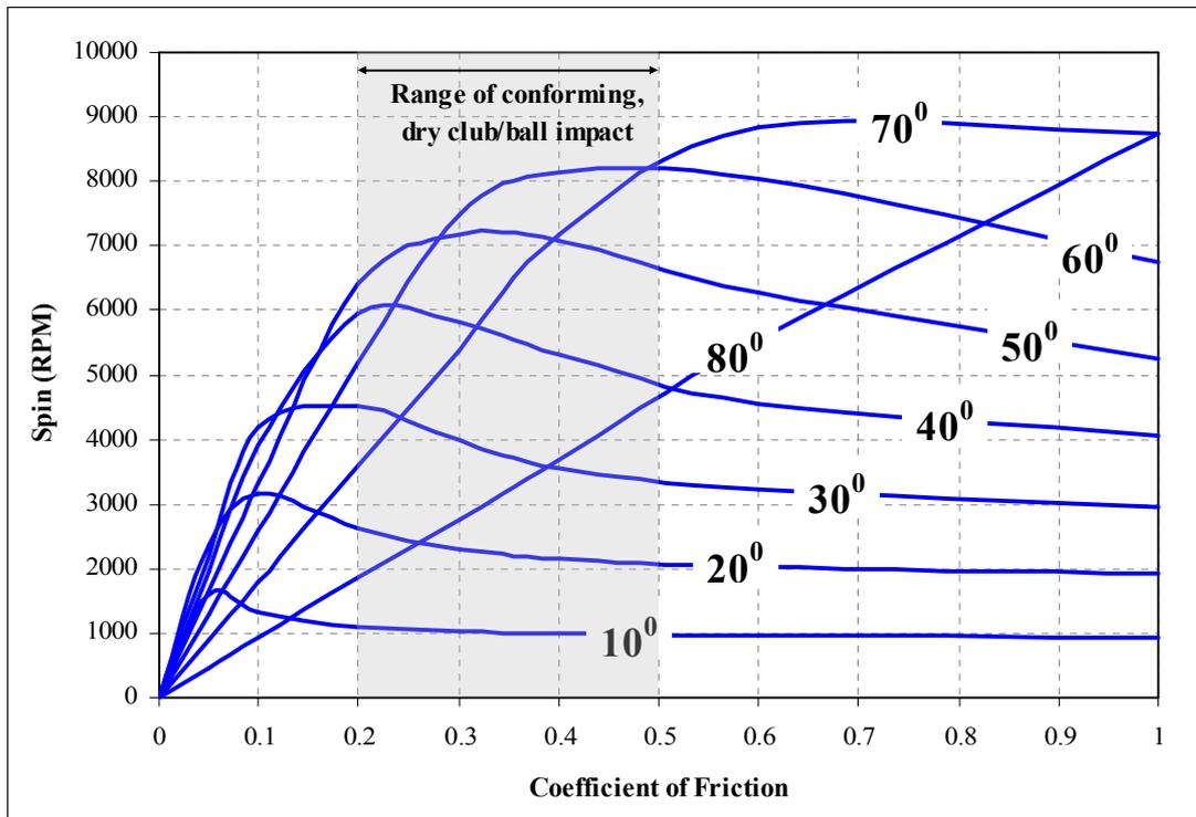
**Figure 10:** Effect of friction on model results for Pinnacle Gold (80 ft/s impact speed)
