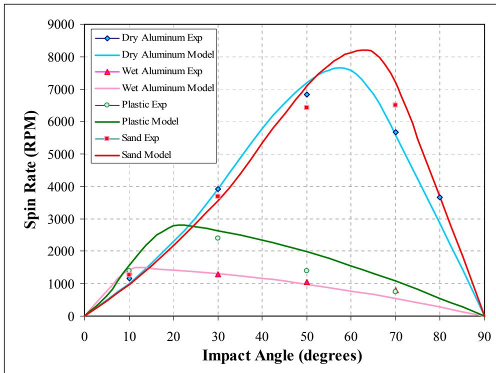
**Figure 7:** Experimental and simulation results for Pinnacle Gold (80 ft/s impact speed)
