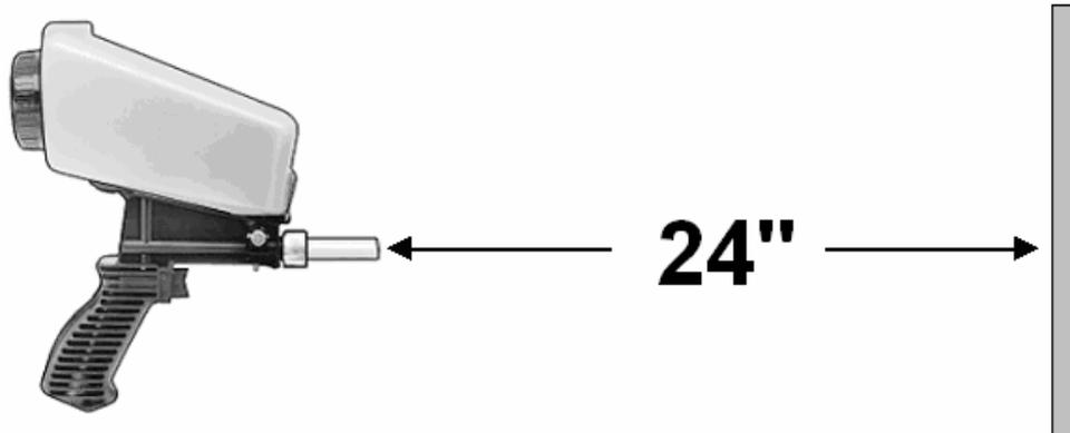
**Figure 4.4:** Abrasive blasting schematic
