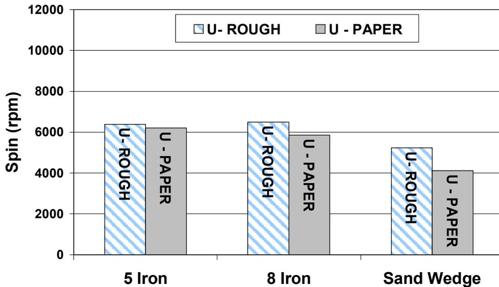
**Figure 9**– Comparison of Spins with a Wet Paper Interface and from Light Rough
