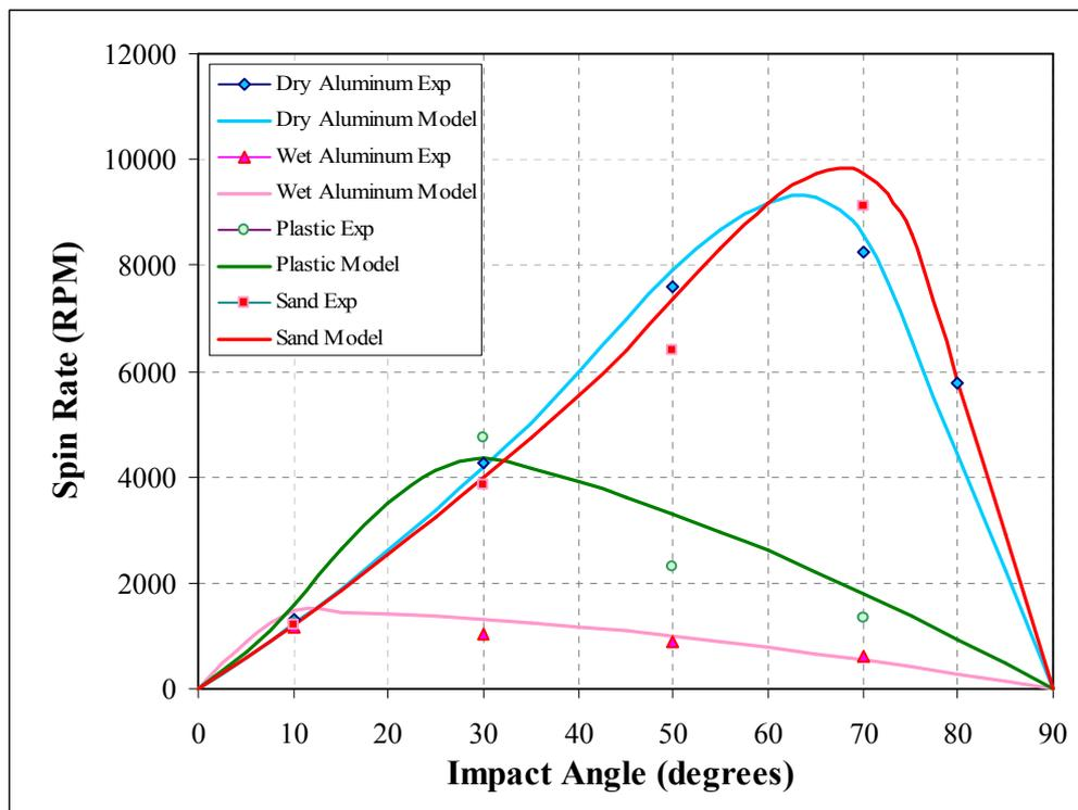
**Figure 8:** Experimental and simulation results for Pro VI (80 ft/s impact speed)
