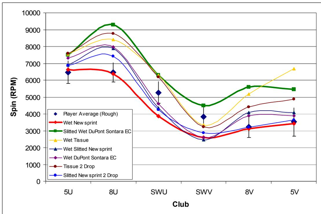
Figure 5.2: Results of various interface material configurations on spin
