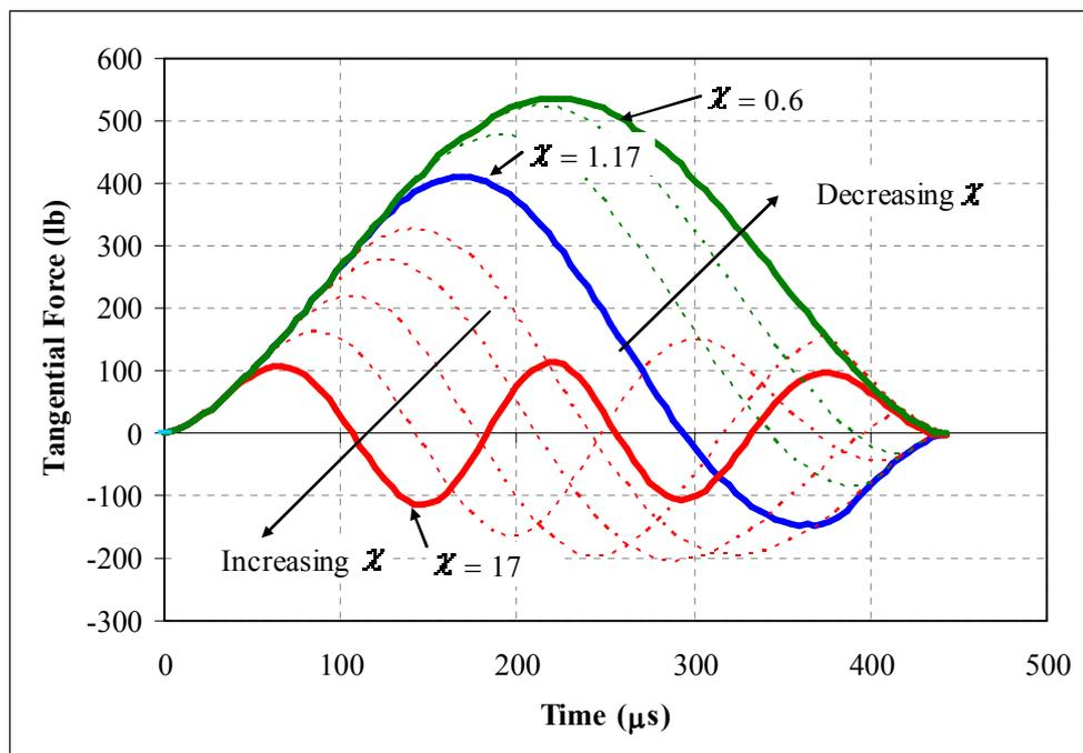
**Figure 3:** Effect of tangential stiffness on tangential force history (30° barrier, 80 ft/s,  $\mu = 0.3$ )
