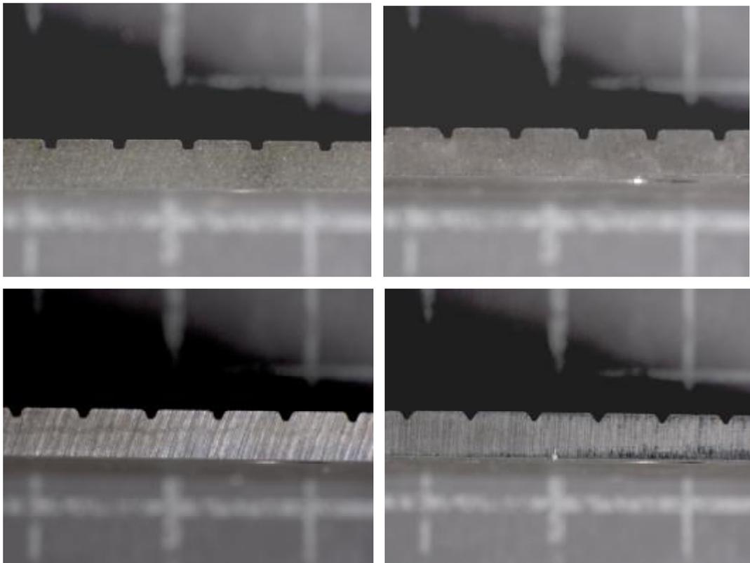
**Figure 6.1:** Cross section of grooved test plates (B-series shown)
