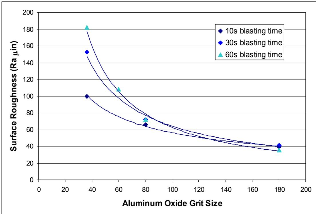
**Figure 3:** Surface roughness as a function of grit size and spray time.
