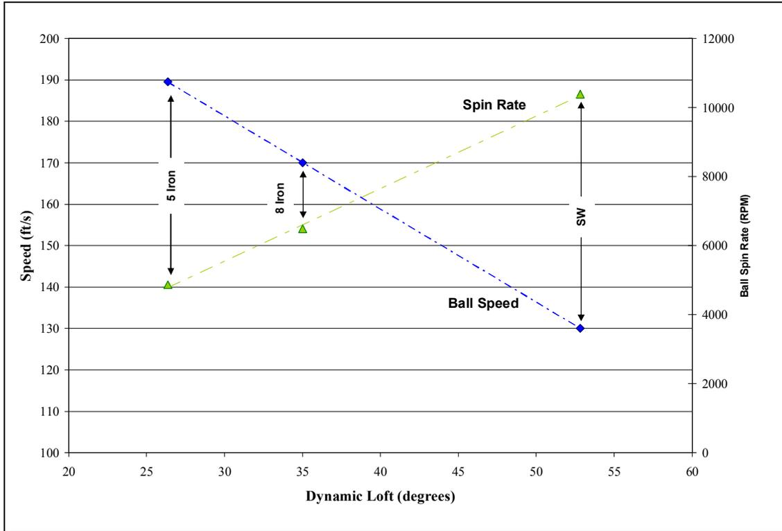
**Figure 1:** Ball speed and spin as a function of dynamic loft
