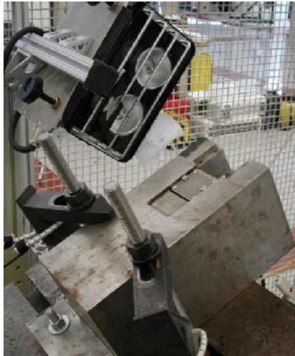
Figure 6.1.2: Grooved test plate oblique impact test setup
